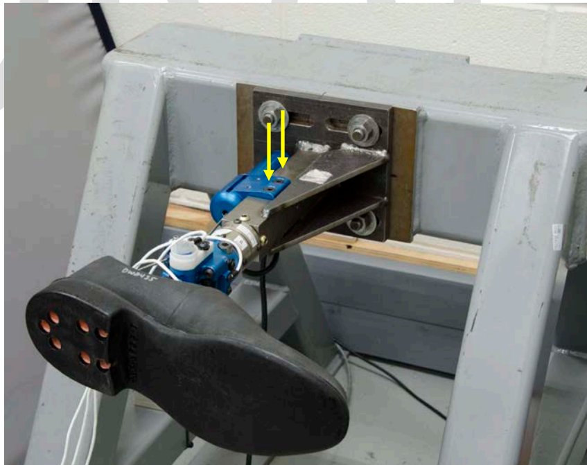
Figure 12-7. Install Achilles tube assembly to mounting bracket
