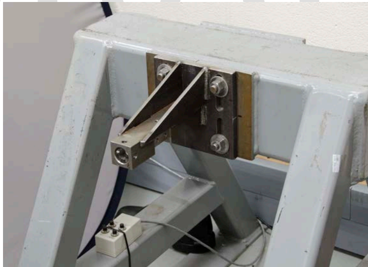
Figure 14-6. Install the lower leg mounting bracket
