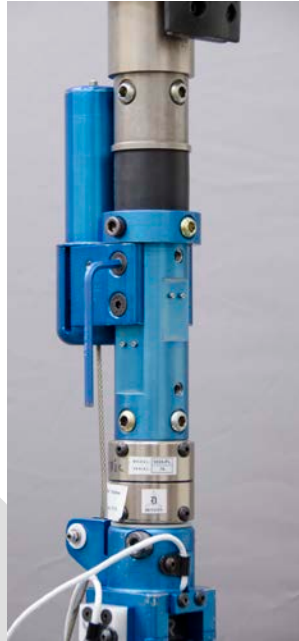
Figure 3-17. Remove Achilles spring tube assembly
