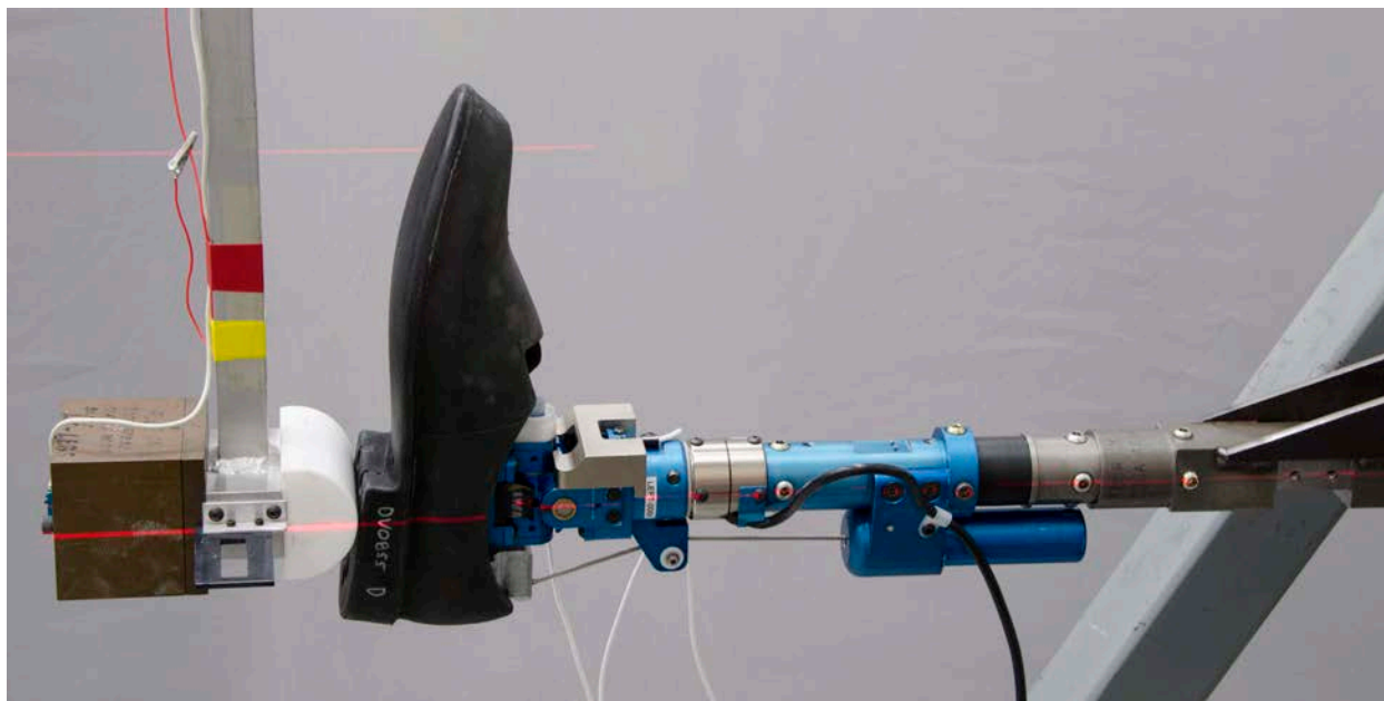
Figure 14-10. Alignment of the impactor for heel impact test
